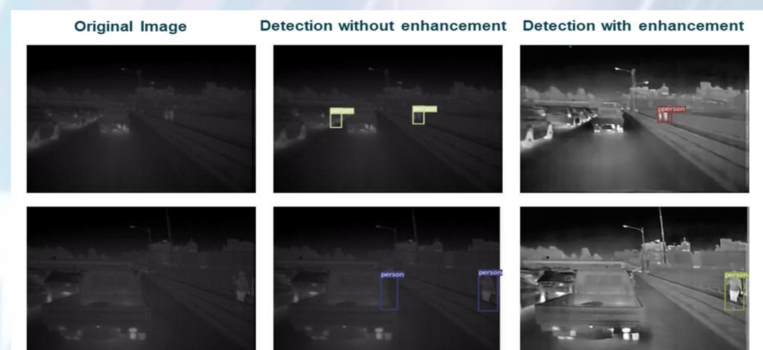
Fig.4: Some results of pedestrian detection using YOLOv3 on thermal images from KAIST dataset with and without TE-GAN enhancement.
